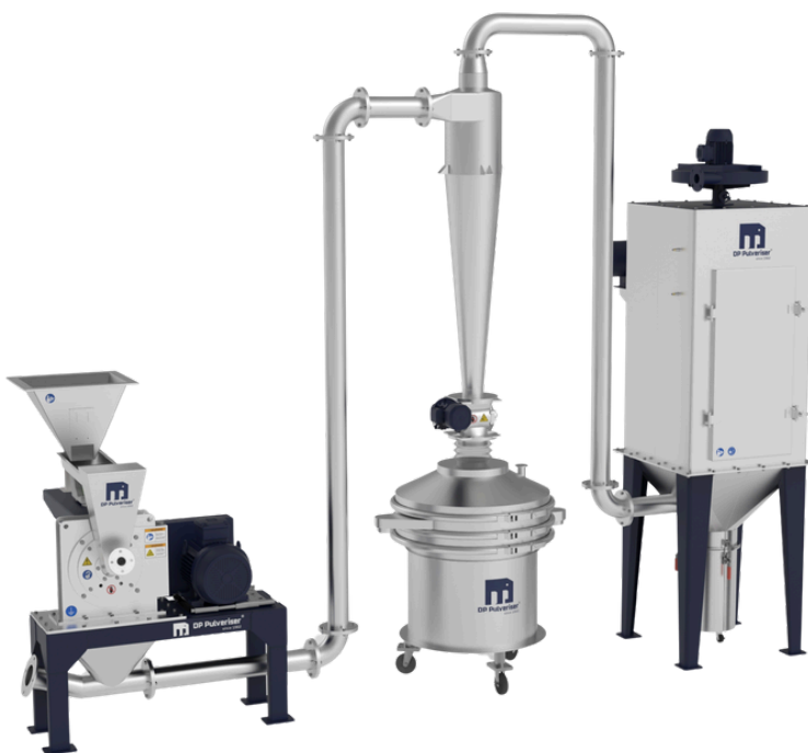
▶ Pneumatic conveying discharge arrangement
